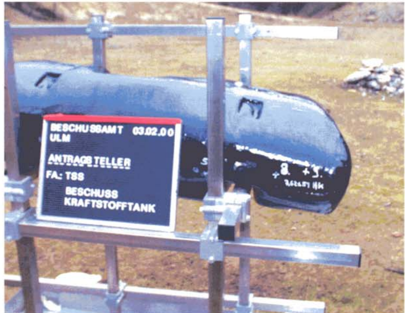
Test sample (front) after the 9 th shot
