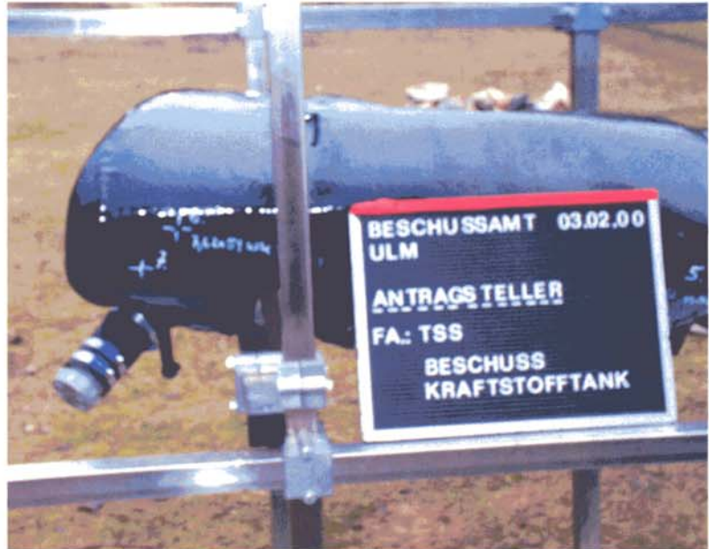
Test sample (rear) after the 7 th shot
