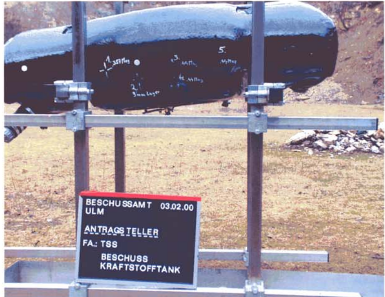
Test sample front after the 5 th shot.
