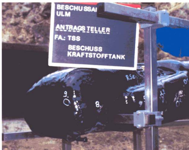
Test sample (rear) after the 9 th shot
